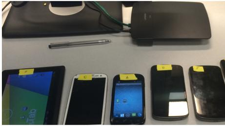
Figure 1: The demo setup includes multiple Android devices and a Wi-Fi router. One device acts as master and rest act as workers.
