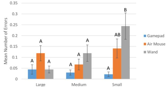
Figure 3: Selection task mean number of errors per trial for each input device per target size. Error bars show standard error. For each target size, levels not connected by the same letter are significantly different.
