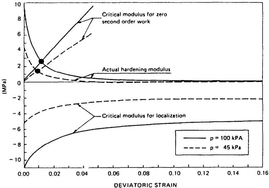
Fig. 2. Critical and actual hardening moduli.  $\sigma_n = 200$  kPa,  $p_n = -0.68$  kPa,  $\alpha = 1.24$ ,  $a = 281$ ,  $G_n = 3333.3$  kPa,  $\chi = -152.71$ ,  $K_n = 21621.00$  kPa. (●) Zero second order work for  $\psi = 16.89$ .
