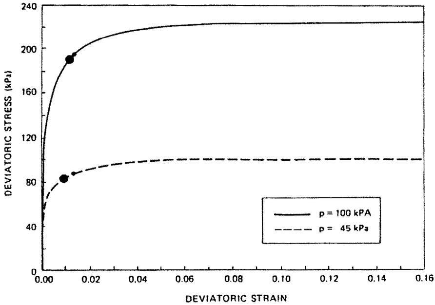
Fig. 4. Deviatoric stress-strain curve.  $\sigma_0 = 200$  kPa,  $p_0 = -0.68$  kPa,  $\alpha = 1.24$ ,  $a = 281$ ,  $G_0 = 3333.3$  kPa,  $\chi = -152.71$ ,  $K_0 = 21621.00$  kPa. (●) Zero second order work for  $\psi = 16.89$ . (●) Zero second order work for  $\psi = 0$  (constant bulk modulus).
