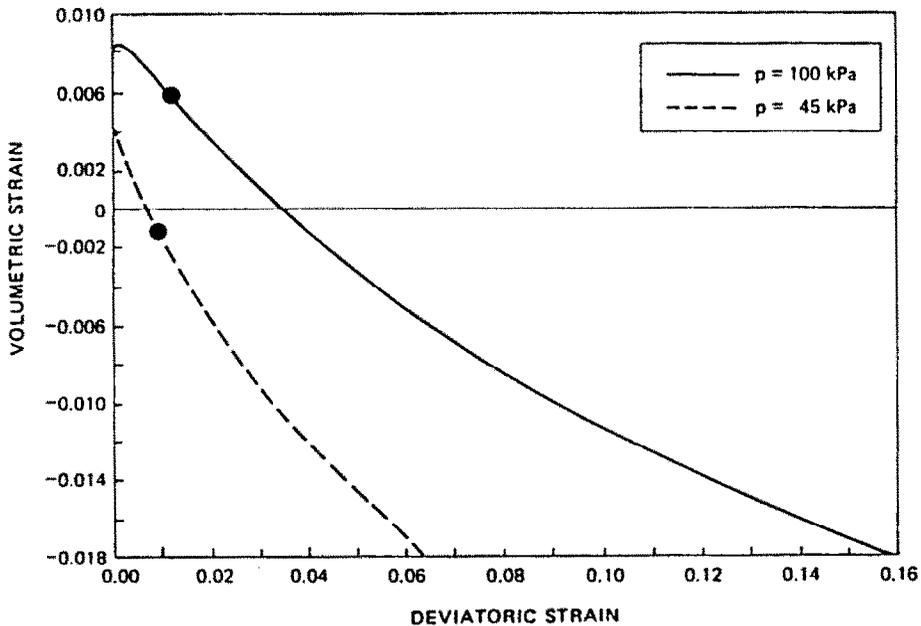
Fig. 5. Volumetric vs deviatoric strain.  $\sigma_0 = 200$  kPa,  $p_0 = -0.68$  kPa,  $\alpha = 1.24$ ,  $a = 281$ ,  $G_0 = 3333.3$  kPa,  $\chi = -152.71$ ,  $K_0 = 21621.00$  kPa. (●) Zero second order work for  $\psi = 16.89$ .
