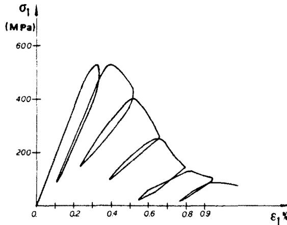
Fig. 1. Uniaxial compression of a rock-like material.
