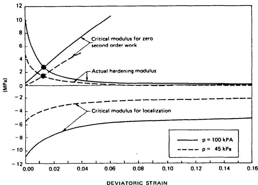
Fig. 3. Critical and actual hardening moduli.  $\sigma_0 = 200$  kPa,  $p_0 = -0.68$  kPa,  $\alpha = 1.24$ ,  $a = 281$ ,  $G_0 = 3333.3$  kPa,  $\chi = -152.71$ ,  $K_0 = 21621.00$  kPa. (●) Zero second order work for  $\psi = 0$  (constant bulk modulus).
