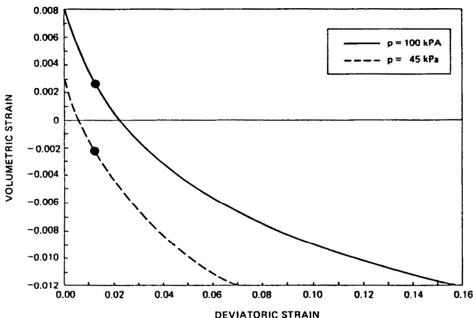
Fig. 6. Volumetric vs deviatoric strain.  $\sigma_0 = 200$  kPa,  $p_0 = -0.68$  kPa,  $\alpha = 1.24$ ,  $a = 281$ ,  $G_0 = 3333.3$  kPa,  $\chi = -152.71$ ,  $K_0 = 21621.00$  kPa. (●) Zero second order work for  $\psi = 0$  (constant bulk modulus).
