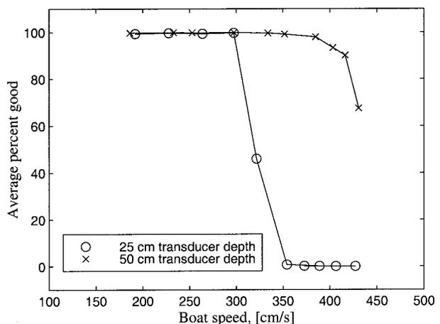
Fig. 4. Comparison of ADCP data quality at different boat speeds and transducer depths.
