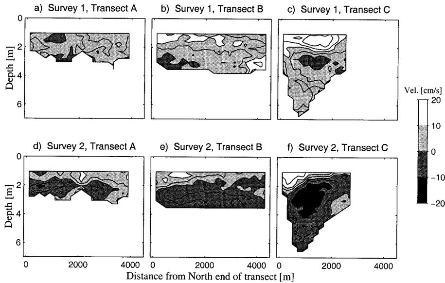
Fig. 5. Along-channel component of rotated ADCP velocities. Flow in the downstream direction is positive; the contour line interval is  $5 \text{ cm s}^{-1}$ .
