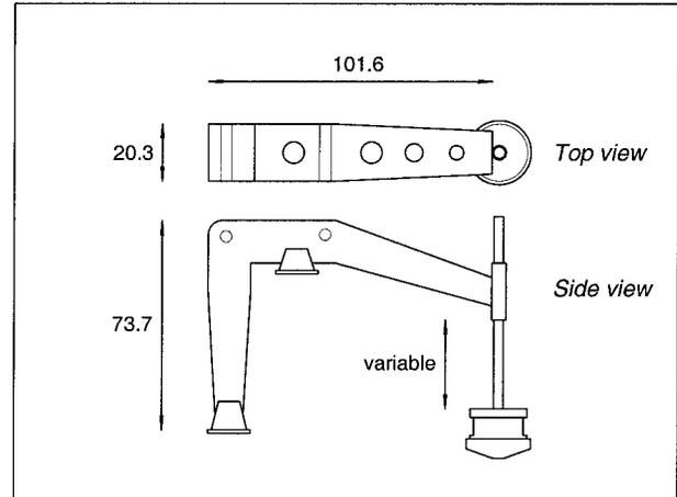
Fig. 1. Schematic drawing of boom design. Dimensions are shown in centimeters.
