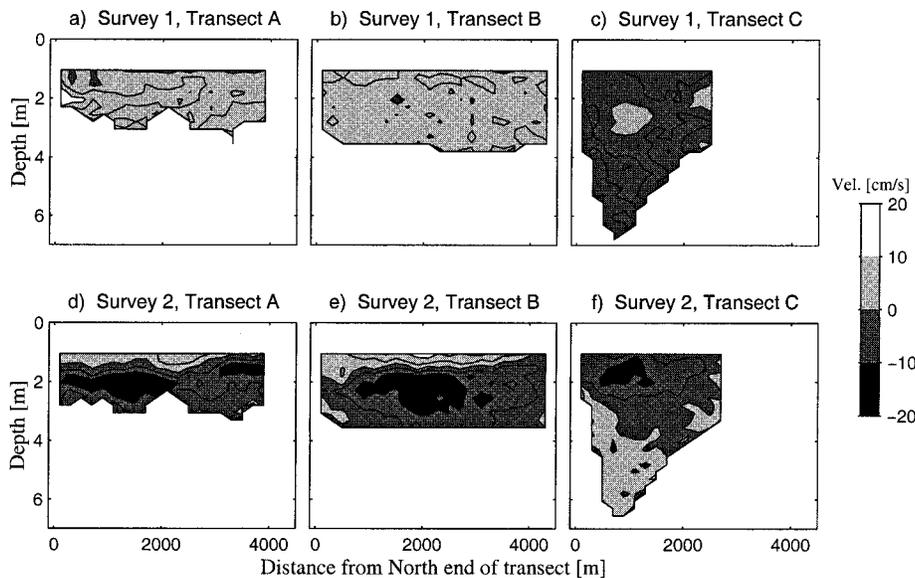
Fig. 6. Cross-channel component of rotated ADCP velocities. Flow toward the north end of each transect is positive; the contour line interval is  $5 \text{ cm s}^{-1}$ .
