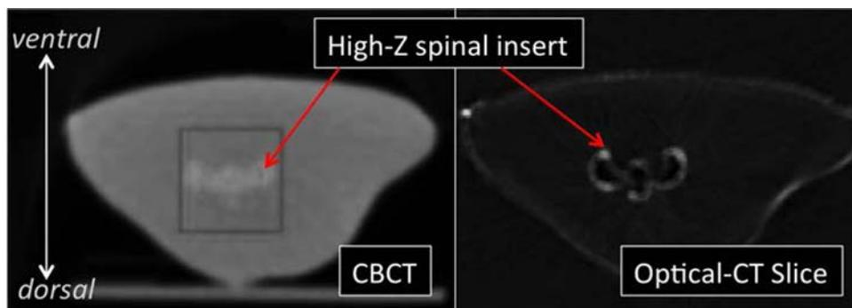
FIG. 6. Visibility of high-Z spinal insert in both CBCT (left) and Optical-CT (right) allows for accurate isocentric targeting.
