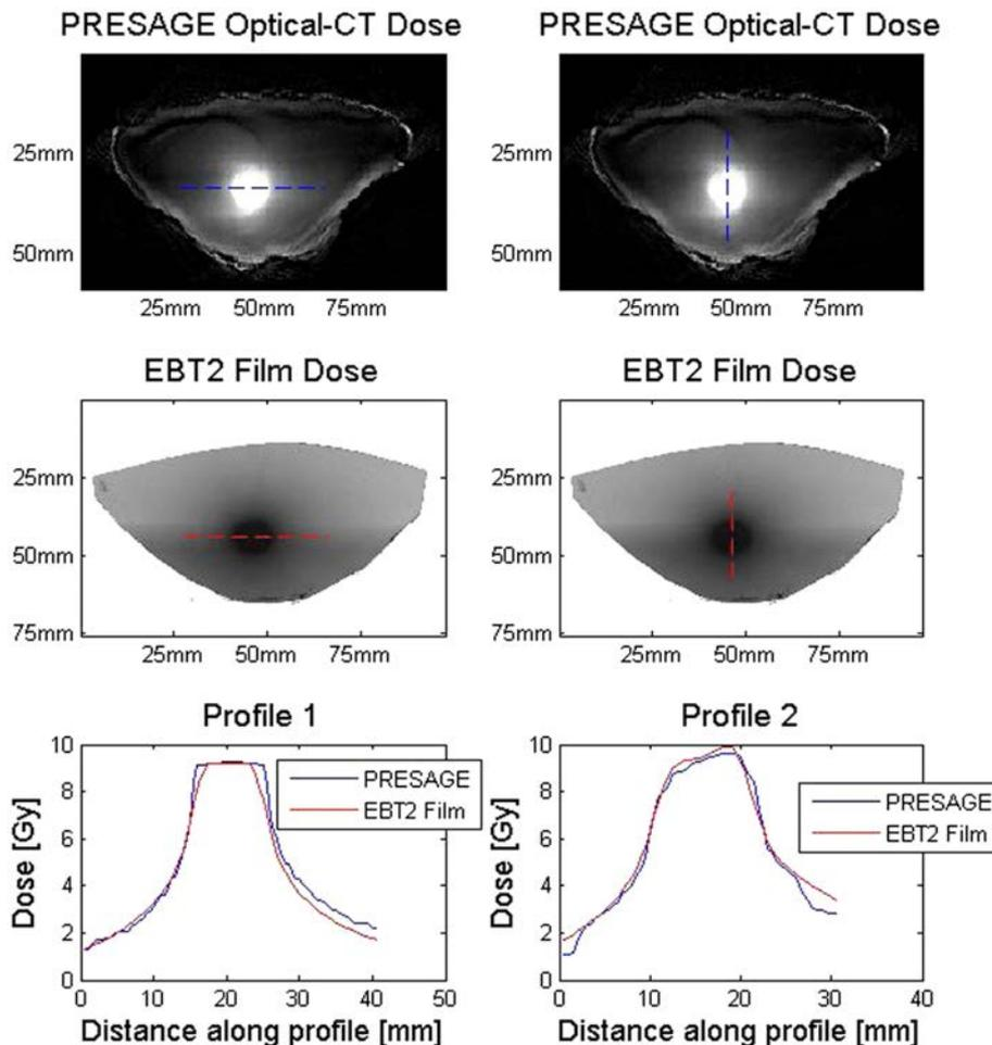
FIG. 9. Axial dose distributions measured with optical-CT (top row) and EBT2 film (middle row), with comparative line profiles (bottom row). Maximum dose/FWHM error was -2.6%/-0.7% for Profile 1 and -2.9%/-1.5% for Profile 2.
