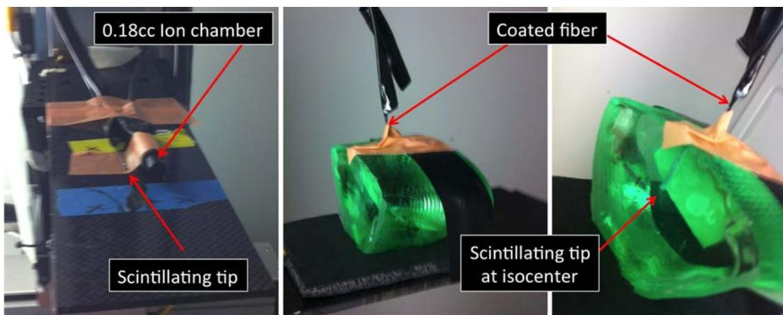
FIG. 4. Setup for absolute dose measurement at isocenter with a novel nanoscintillation detector. First, the detector was calibrated with a RadCal  $0.18 \text{ cm}^3$  ion chamber (left), then, the  $180^\circ$  arc treatment was delivered three times with the scintillating detector placed at the rodent-morphic dosimeter isocenter (center, right).
