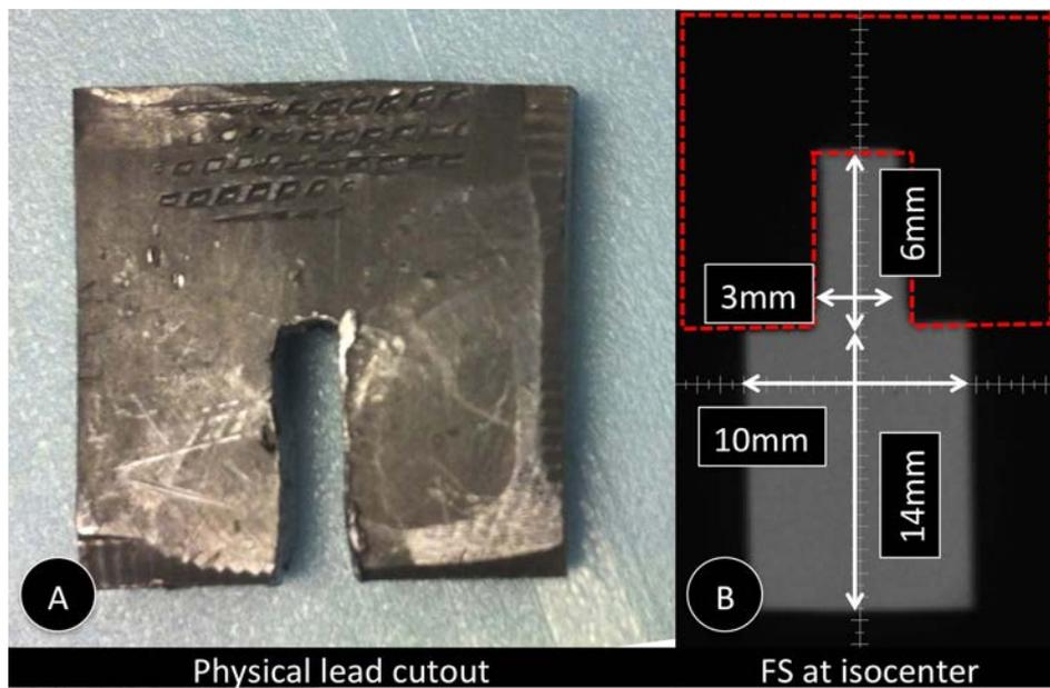
FIG. 3. (A) Lead block (~3 mm thick) cutout used to shape the radiation field into 10 and 3 mm width regions. (B) Radiographic projection image of the field at isocenter (dashed red lines indicate approximate block location).
