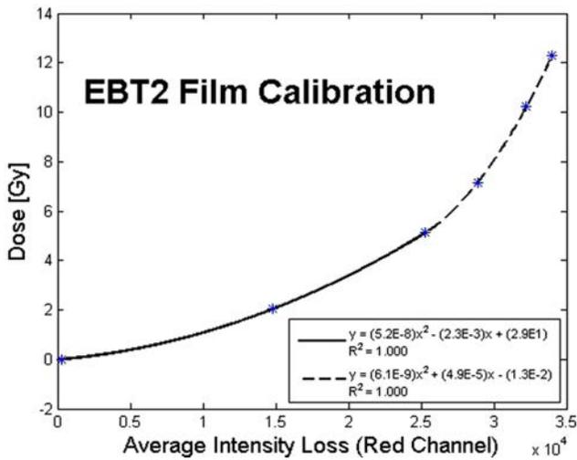
FIG. 8. Biquadratic fit of radiochromic film used for absolute dose verification.
