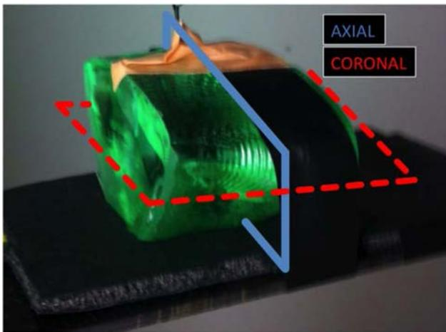
FIG. 5. Schematic showing placement of radiochromic film in axial (solid blue line) and coronal (dashed red line) planes for independent measurement of dose distributions.
