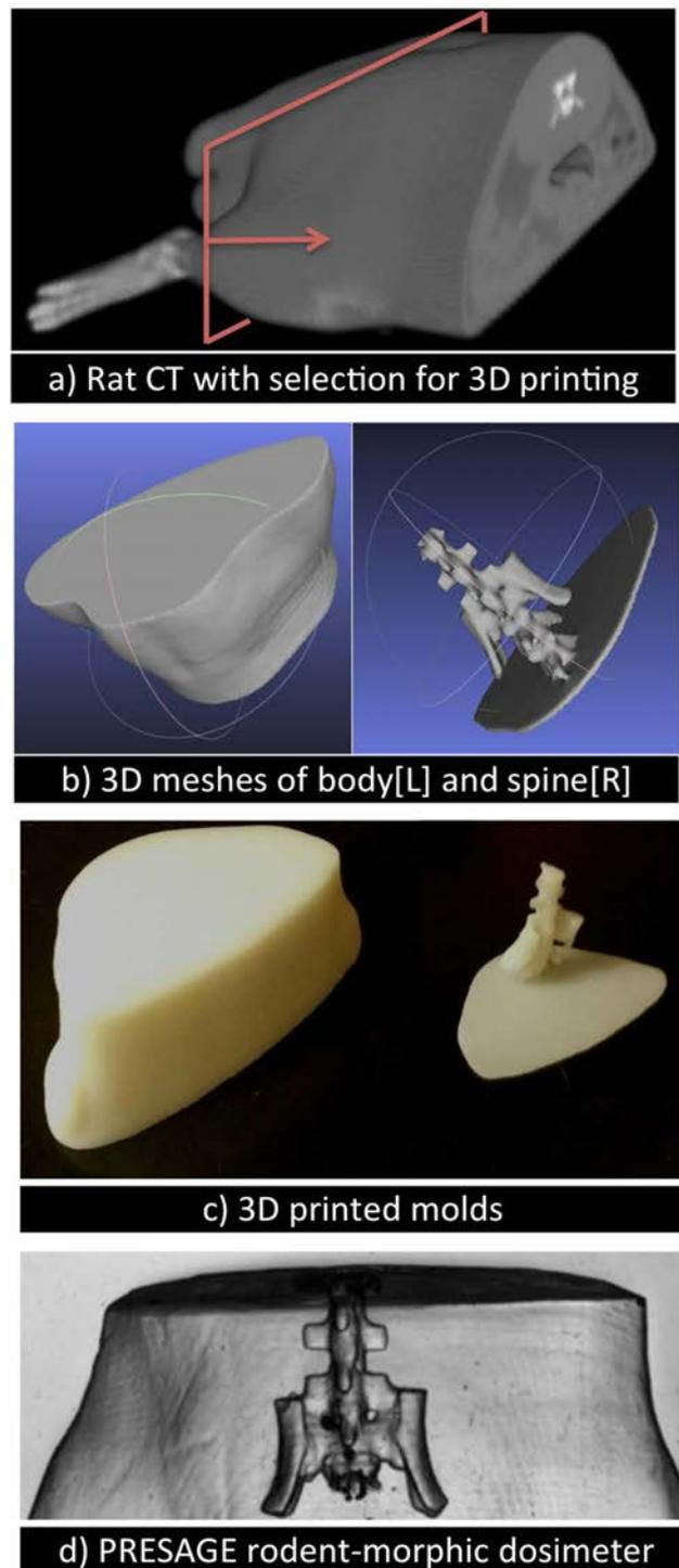
FIG. 1. Illustration of workflow for producing rodent-morphic dosimeters from CT data. Rodent CT data (a) are converted to 3D meshes (b) for printing 3D positive molds (c), which are used to make negative molds for constructing Presage dosimeters [(d)—optical-CT projection shown to highlight spinal insert].
