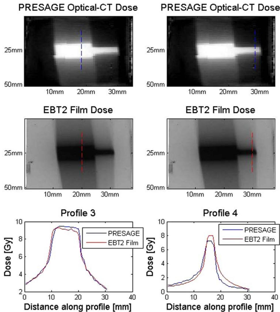
FIG. 10. Coronal dose distributions measured with optical-CT (top row) and EBT2 film (middle row), with comparative line profiles (bottom row). Maximum dose/FWHM error was 1.6%/–0.5% for Profile 3 and –6.7%/4.4% for Profile 4.
