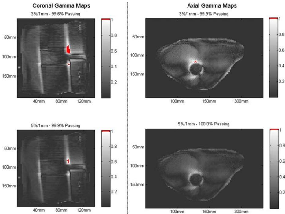
FIG. 11. Gamma maps comparing axial and coronal 2D Presage and film distributions at 1 mm distance-to-agreement 3% and 5% dose difference thresholds. Failing pixels accentuated for easy visualization.
