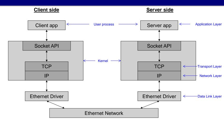
• Client and Server communicating across Ethernet using TCP/IP
