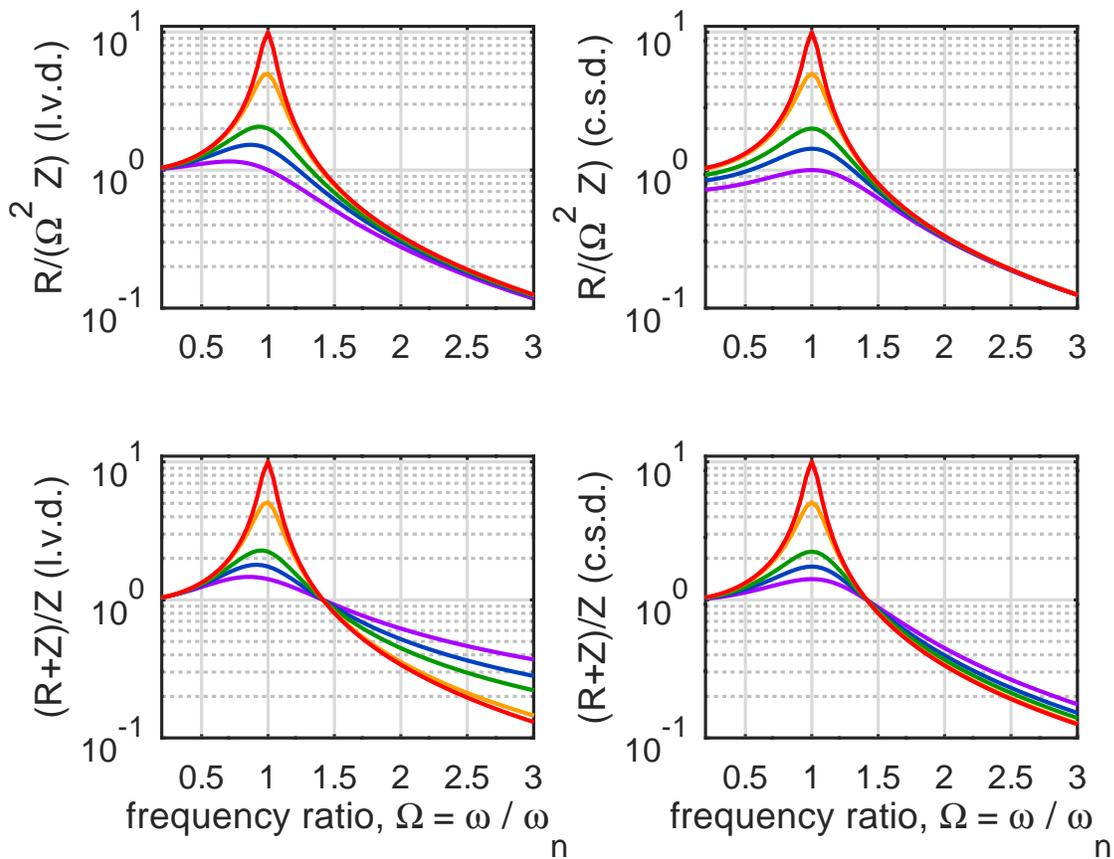
Figure 2. Magnitude of Compliance (top) and Transmissibility (bottom) of inertially-driven oscillators with linear viscous damping (left) and complex-stiffness damping (right).  $\xi = 0.1, 0.2, 0.5, 0.7, 1.0$  and  $\zeta = 0.05, 0.10, 0.25, 0.35, 0.50$ . For comparable suppression of resonant responses, the complex stiffness damping model attenuates the high frequency transmissibility more than the linear viscous damping does.
