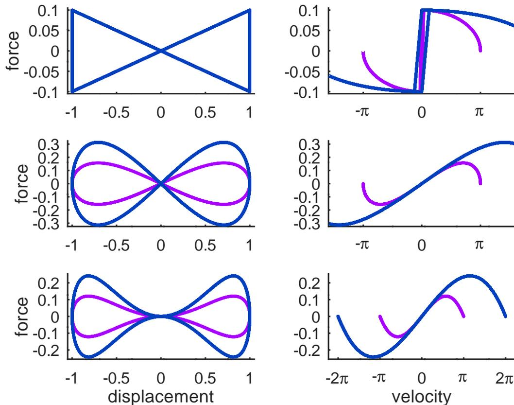
Figure 1. Force-displacement and force-velocity relationship for complex-stiffness damping (equations (2), (3), and (4), sometimes called “butterfly damping”) for  $\omega = \pi$  (violet) and  $\omega = 2\pi$  (blue) and  $\xi = 0.1$ .
