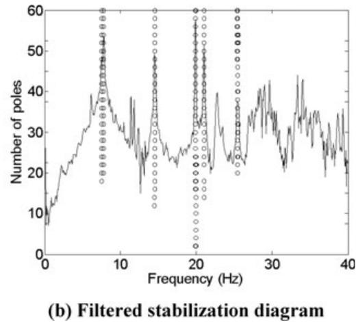
Fig. 5: Stabilization diagrams
