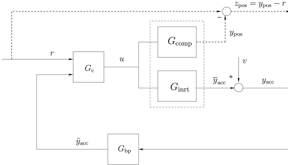
**Fig. 2 Control architecture for discrete-time LQG position control using acceleration feedback and a backward-path controller  $G_{bp}$**
