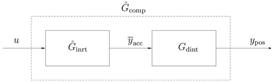
**Fig. 3 Construction of the compliance  $\hat{G}_{\text{comp}}$  by cascading a double integrator with the identified inertia**
