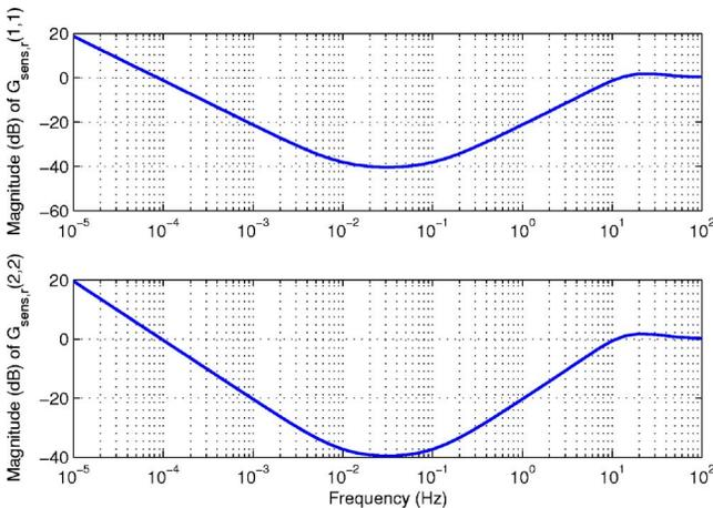
**Fig. 11** Magnitudes of the diagonal entries of  $G_{sens,r}$ , the sensitivity transfer function between the reference position command  $r$  and the position-tracking error  $z_{pos}$ . The magnitude of the sensitivity function is low in the required bandwidth between 0.1 Hz and 1 Hz.
