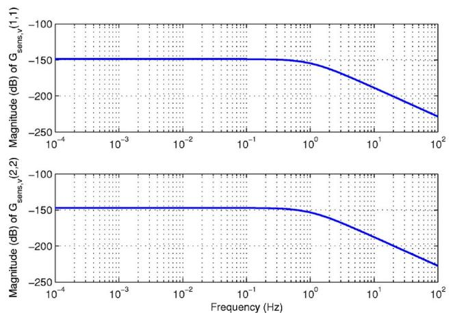
**Fig. 12** Magnitudes of the diagonal entries of  $G_{sens,v}$ , the sensitivity function between the bias  $v$  and position-tracking error  $z_{pos}$ . The inclusion of a backward-path controller with zero dc gain ensures that as  $k \rightarrow \infty$  the position-tracking performance is not affected by the sensor bias  $v$ .
