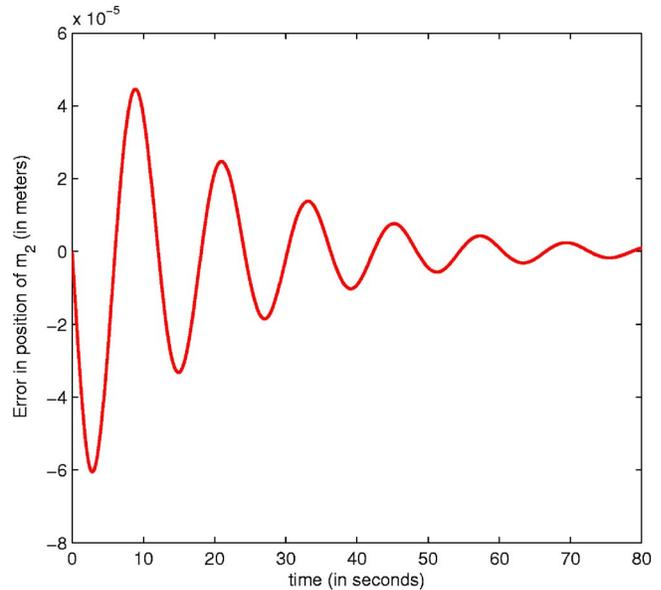
Fig. 6 Error between the position of  $m_2$  and the output  $y_{\text{pos},2}$  from the identified compliance model when  $u_1=0$  and  $u_2$  is an impulse
