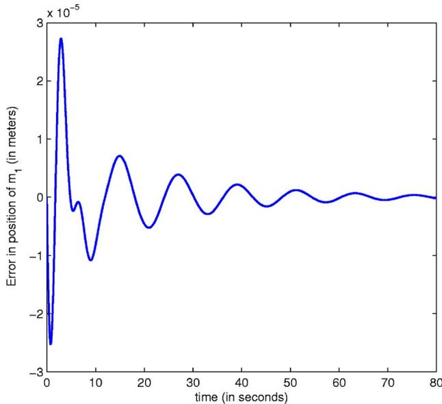
Fig. 5 Error between the actual position of  $m_1$  and the output  $y_{\text{pos},1}$  of the identified compliance model when  $u_1$  is an impulse and  $u_2=0$ . For position-tracking controller synthesis, the identified compliance is used.
