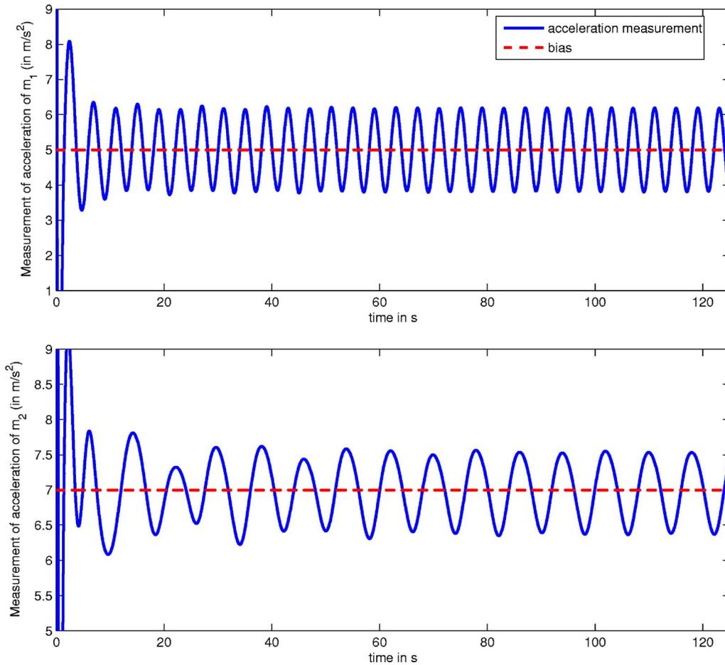
**Fig. 10** Acceleration measurements of the two masses. The sensor biases in the accelerometers are shown as dashed lines.
