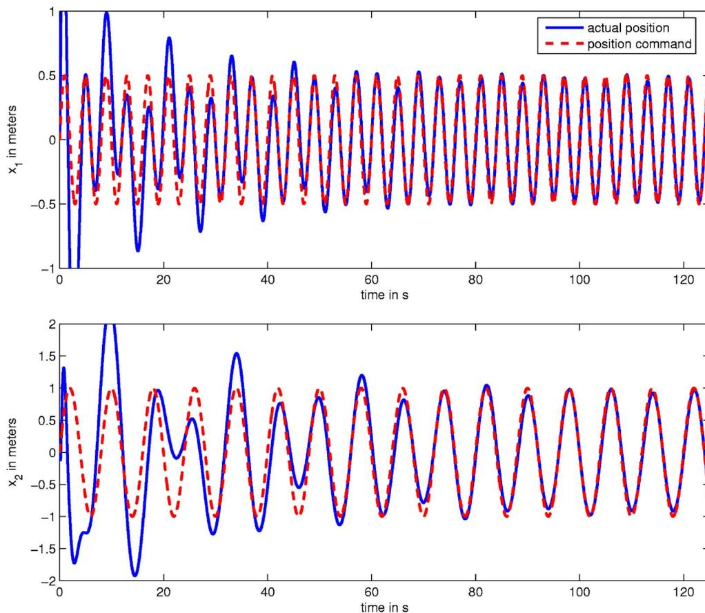
Fig. 9 Position-command following for the two-mass system using an LQG controller and a backward-path controller. The LQG controller  $G_c$  produces the control input  $u$  to track the position command  $r$ , while the backward-path controller with zero dc gain, that is, a zero at  $z=1$ , rejects the sensor bias.
