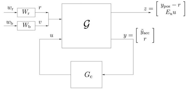
**Fig. 1 Standard problem for designing a position-tracking controller  $G_c$  that uses biased acceleration measurements. To facilitate controller synthesis using LQG, the backward-path controller  $G_{\text{bp}}$  that is used to reject the sensor bias is included in the Plant  $\mathcal{G}$ .**
