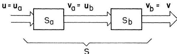
FIG. 3. Cascade connection of  $S_a$  followed by  $S_b$
