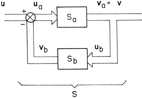
FIG. 4. Feedback system  $S$  with  $S_a$  in the forward path and  $S_b$  in the return path
