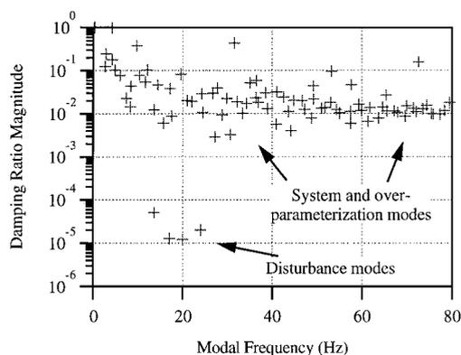
Fig. 4 Modal damping vs modal frequency,  $p = 90$ .
