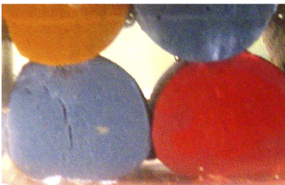
Fig. 5. Dissolution and damage at the chalk contact after 64 h.
