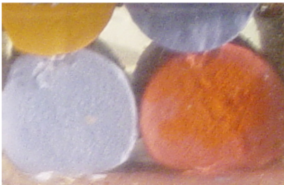
Fig. 4. Dissolution and damage at the chalk contact after 24 h.
