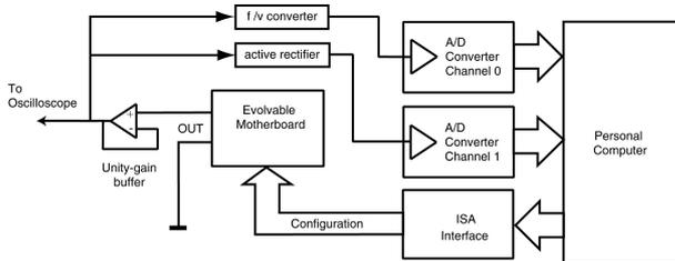
Figure 2: the oscillator experimental setup
