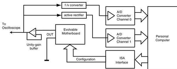
Figure 2: the oscillator experimental setup
