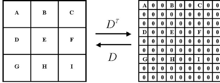
Fig. 3. Effect of upsampling  $D^T$  matrix on a  $3 \times 3$  image and downsampling matrix  $D$  on the corresponding  $9 \times 9$  upsampled image (resolution enhancement factor of three). In this figure, to give a better intuition, the image vectors are reshaped as matrices.
