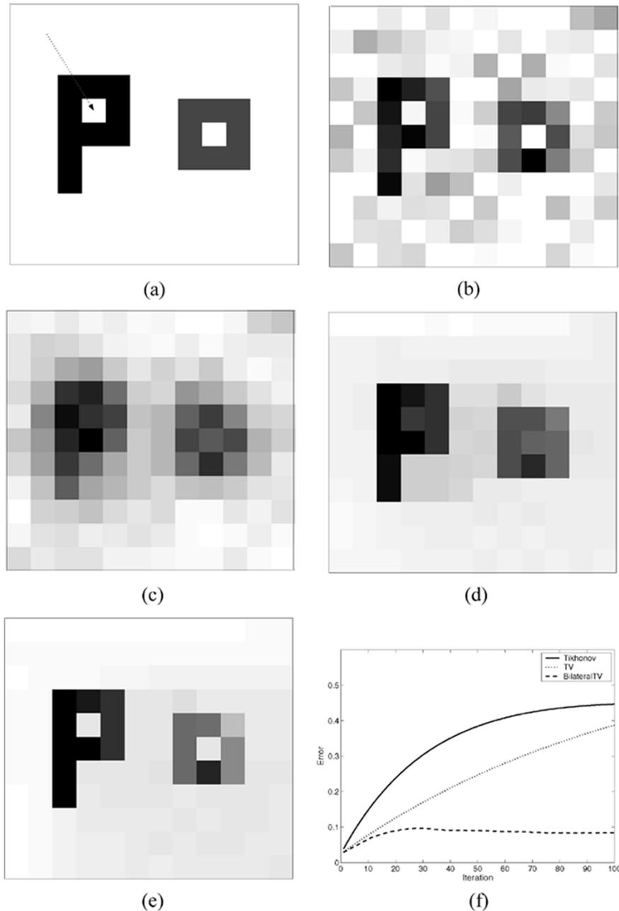
Fig. 4. (a)-(e) Simulation results of denoising using different regularization methods. (a) Original. (b) Noisy. (c) Reconstruction using Tikhonov. (d) Reconstruction using TV. (e) Reconstruction using bilateral TV. (f) Error in gray-level value estimation of the pixel indicated by arrow in (a) versus the iteration number in Tikhonov (solid line), TV (dotted line), and bilateral TV (broken line) denoising.
