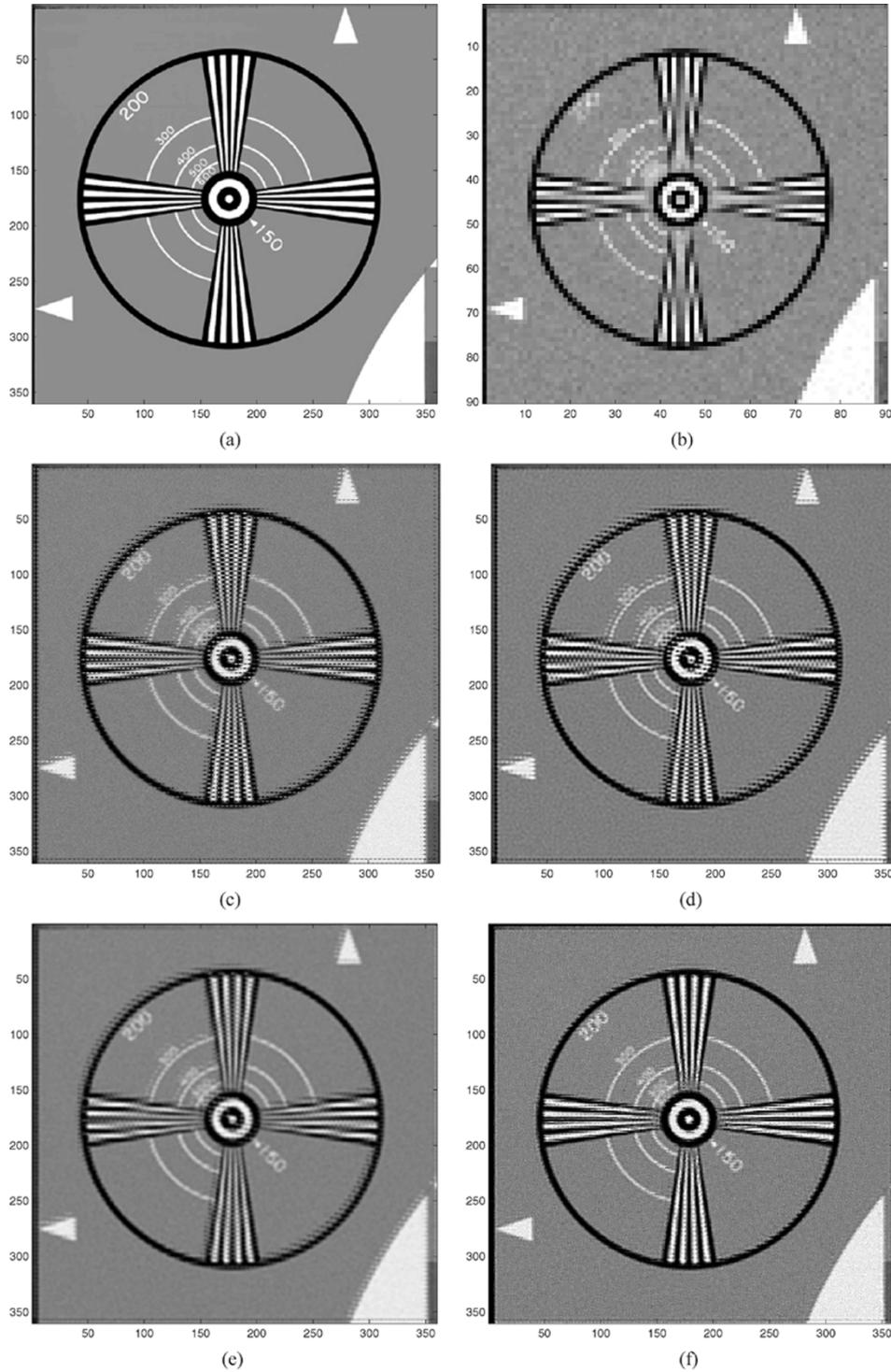
Fig. 9. Simulation results of different resolution enhancement methods are applied to the (a). (a) Original HR frame. (b) LR frame. (c) Shift and add result [5]. (d) Deconvolved shift and add [5]. (e)  $L_2 +$  Tikhonov. (f) Zomet method [14].
