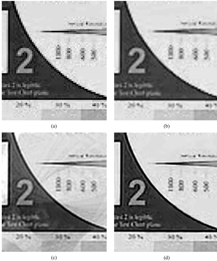
Fig. 11. Results of different resolution enhancement methods applied to ADYORON test sequence. (a) One of 20 LR frames. (b) Cubic spline interpolation. (c)  $L_2 +$  Tikhonov. (d)  $L_1 +$  bilateral TV.
