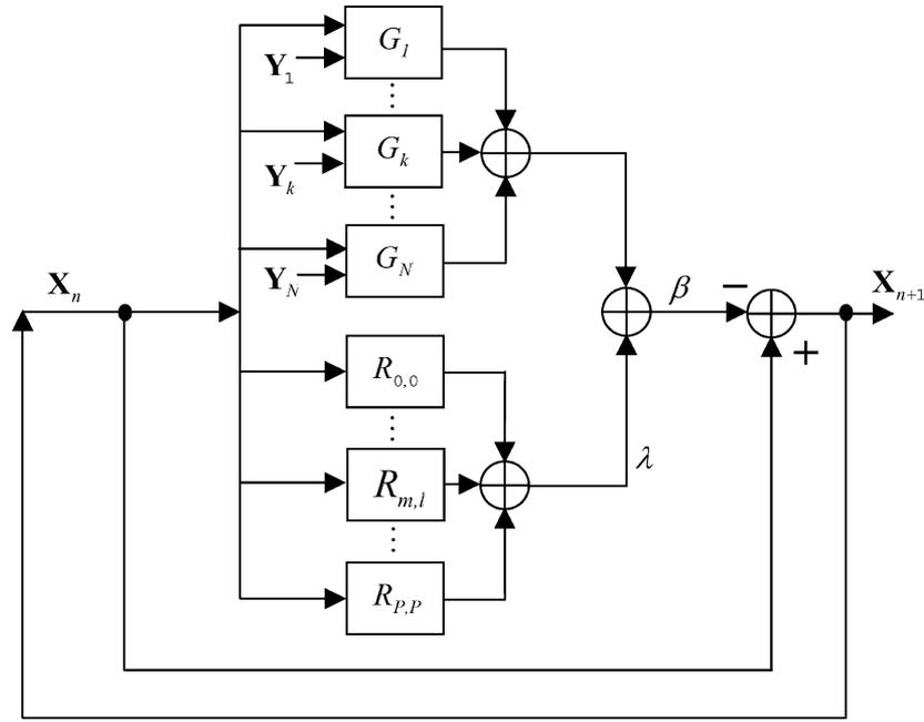
Fig. 6. Block diagram representation of (22), blocks  $G_k$ , and  $R_{m,l}$  are defined in Fig. 7.
