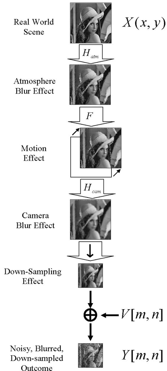
Fig. 1. Block diagram representation of (1), where  $X(x, y)$  is the continuous intensity distribution of the scene,  $V[m, n]$  is the additive noise, and  $Y[m, n]$  is the resulting discrete low-quality image.
