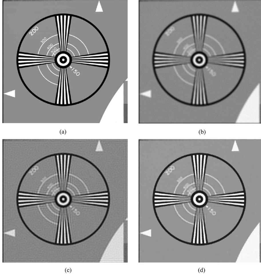
Fig. 5. Simulation results of deblurring using different regularization methods. The mean square error (MSE) of reconstructed image using Tikhonov regularization (c) was 313. The MSE of reconstructed image using bilateral TV (d) was 215. (a) Original. (b) Blurred and noisy. (c) Best Tikhonov regularization. (d) Proposed regularization.
