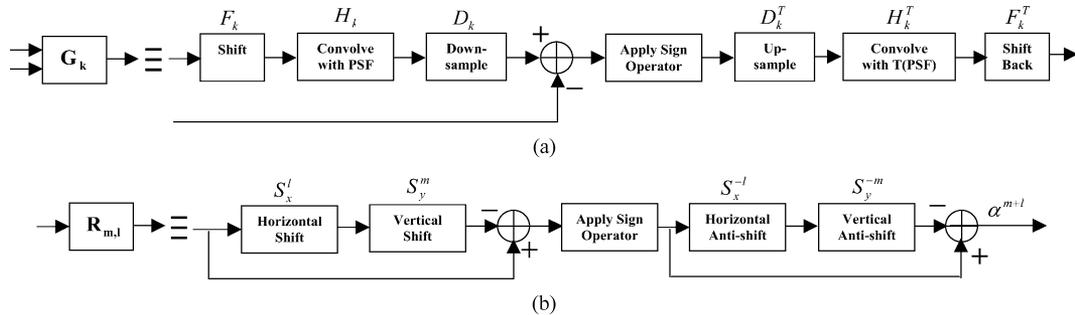
Fig. 7. Extended block diagram representation of  $G_k$  and  $R_{m,l}$  blocks in Fig. 6. (a) Block diagram representation of similarity cost derivative ( $G_k$ ). (b) Block diagram representation of regularization cost derivative.
