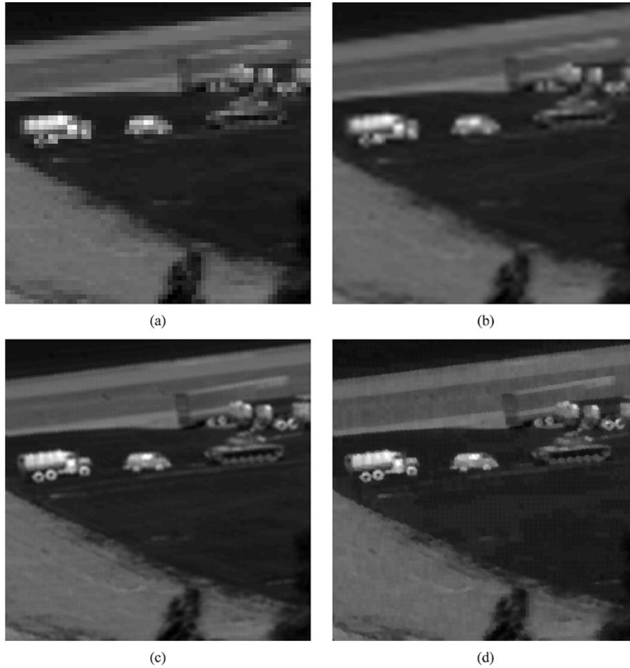
Fig. 10. Results of different resolution enhancement methods applied to Tank sequence. (a) One of eight LR frames. (b) Cubic spline interpolation. (c)  $L_2$  + Tikhonov. (d)  $L_1$  + bilateral TV.
