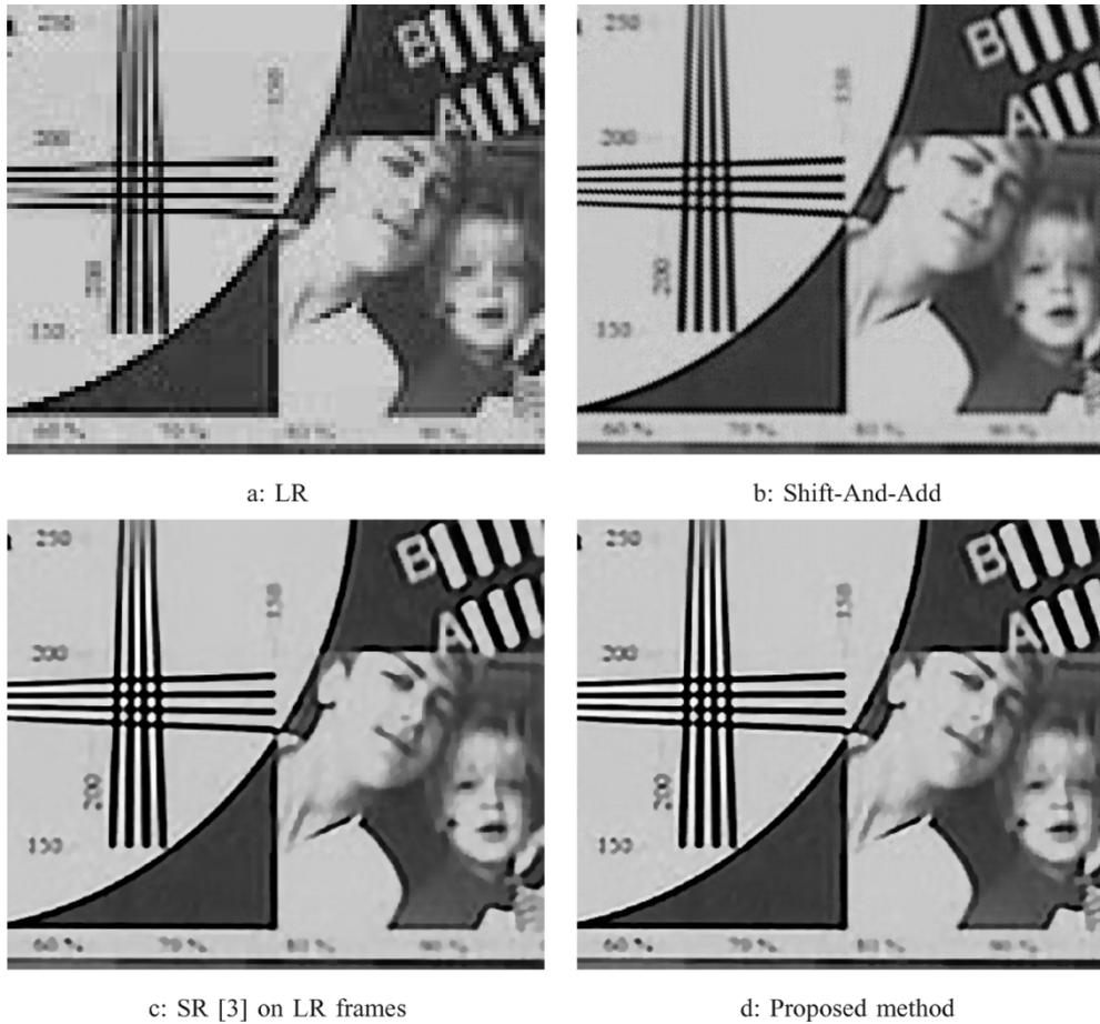
Fig. 9. Multiframe color super-resolution implemented on a real data sequence. (a) One of the input LR images and (b) the shift-and-add result increasing resolution by a factor of 4 in each direction. (c) Result of the individual implementation of the super-resolution [3] on each color band. (d) Implementation of (15) which has increased the spatial resolution, removed the compression artifacts, and also reduced the color artifacts. These images are zoomed in Fig. 10.
