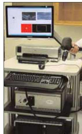
Figure 4. The Bioptigen handheld SD OCT scanner.
