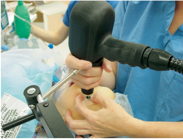
FIGURE 1. Photograph showing the hand-held spectral-domain optical coherence tomography (SD OCT) being used to image an infant eye. The infant is supine and under endotracheal anesthesia. The imaging hand piece is held over the infant's eye while the SD OCT output is observed on a computer screen on an adjacent wheeled cart.
