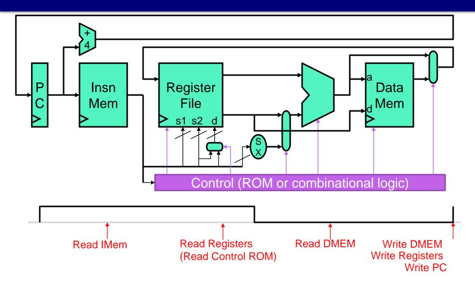
How do we sub-divide timing like this? *Pipelining!* (Covered later)
