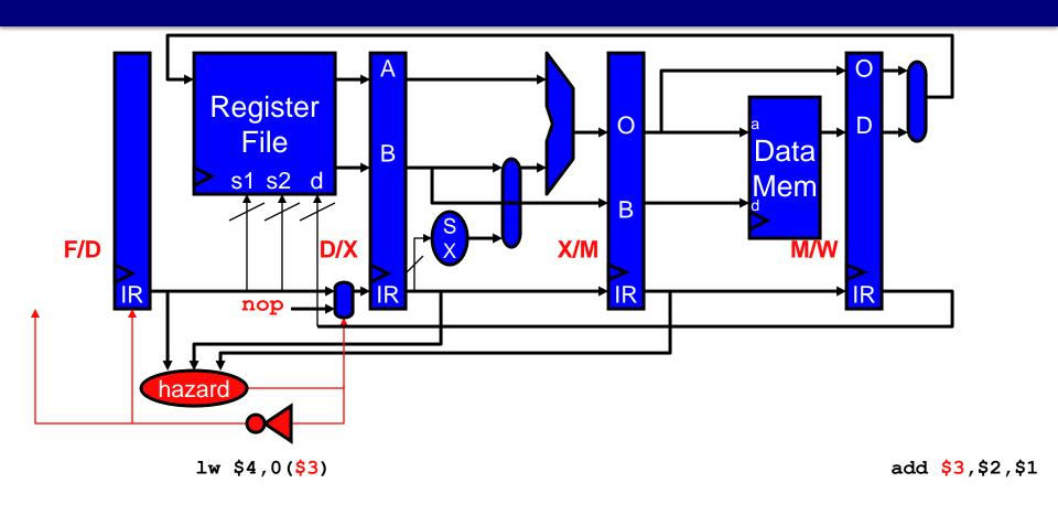
(F/D.IR.RS1 == D/X.IR.RD) || (F/D.IR.RS2 == D/X.IR.RD) || (F/D.IR.RS1 == X/M.IR.RD) || (F/D.IR.RS2 == X/M.IR.RD) = **0**
