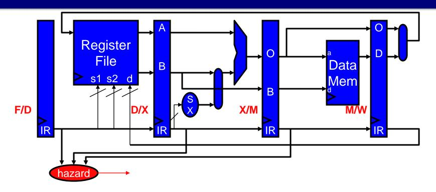
Compare F/D insn input register names with output register names of older insns in pipeline
