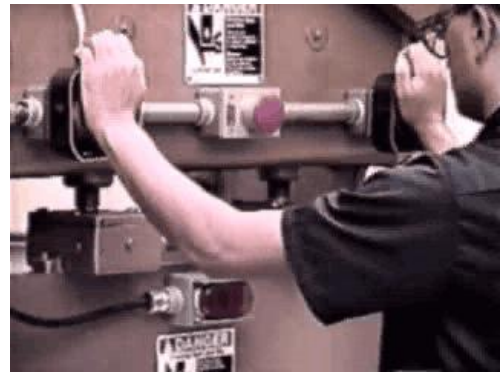
A two-handed, non-repeating industrial press. See here for animated version.
