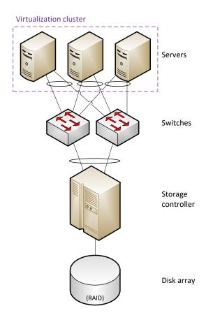
The virtualization cluster is running load-balancing and high availability clustering software, allowing automatic migration of VMs. When balanced, average utilization of each of the servers is around 75%.
