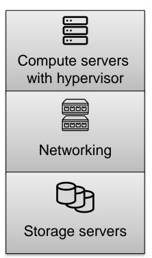
**Aggregate**: Cluster disk-less interchangeable servers **Separate**: Run virtual machines (VMs) that can freely migrate
