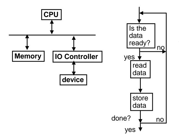
busy wait loop not an efficient way to use the CPU unless the device is very fast!
