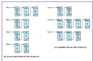
Figure 4.2 Example of Access Control Structures
